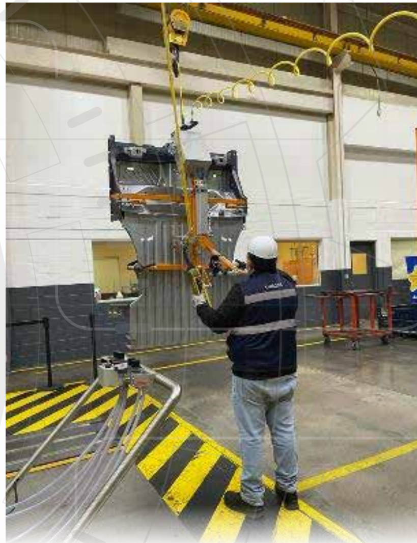
Lift Assist de pisos traseros Maverick Sonora Forming
